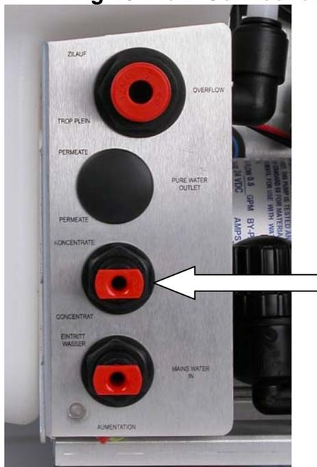
Using an 8mm stem elbow push the plain stem part into the "**Drain**" port. Then into the elbow, push in one end of a length of 8mm tubing. Run the tubing to a suitable drain, within 2 meters of the unit ensuring the tubing is unrestricted and does run more than 1 meter above the unit
