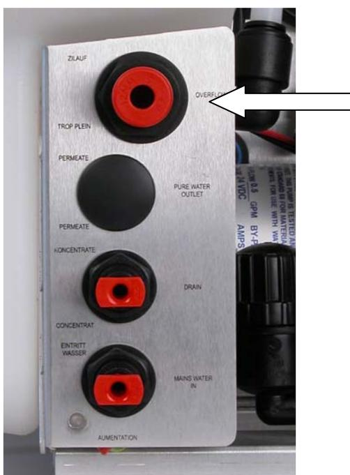
Using a 12mm Stem elbow supplied, push the plain stem end into the "**Overflow**" connection on the rear of the unit. To the female end of the elbow, push in a length of the 12mm tubing. Run the tubing to a suitable drain, within 2 meters of the unit, ensuring the tubing is unrestricted.
